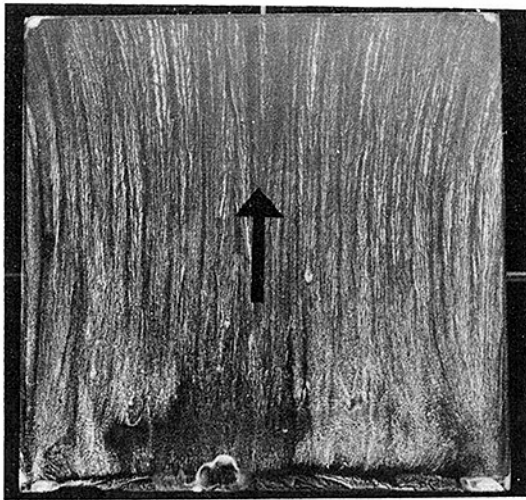
Fig. 7 Undersurface flow pattern on a cube with a ground clearance of 0.056c and with the floor moving.
